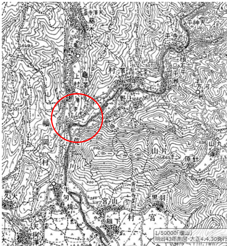
図1 吉沢・牛句付近の河道は亀沢川合流部の上流左岸で水衝部に淵が形成 (明治43年) Figure 1: A pool formed at the water collision point on the left bank upstream of the confluence of the Kamezawa River near Kissawa and Ushiku (1910 Meiji43)
